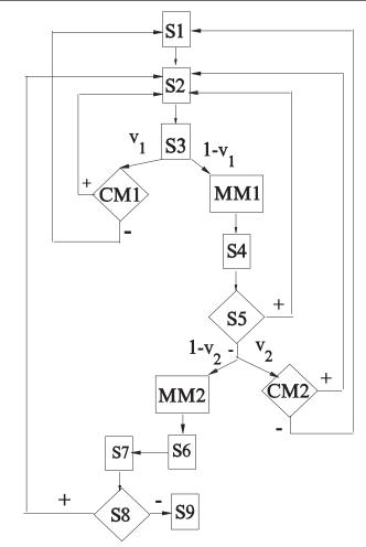
**Figure 1.** The program of performing quantum dialogue protocol. The sign '+' implies passing the control, while the sign '-' implies that the condition under control is not satisfied.  $v_1$ ,  $1 - v_1$ ,  $v_2$  and  $1 - v_2$  indicate probabilities of corresponding choice for a message mode or a control mode. For contents of the boxes see the text.
