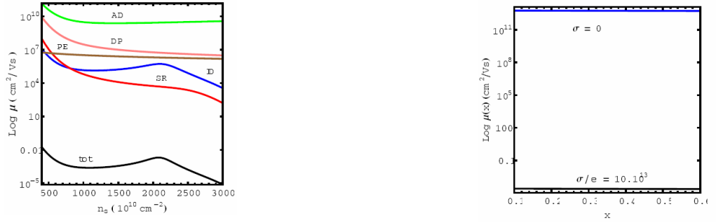
Fig. 2. 2DEG mobility of an UID \text{GaN}/\text{AlGaN} SFQW vs. sheet electron density n_s and vs. an Al content x .
