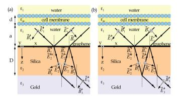
FIG. 1. Schematic picture of a lipid membrane and graphene on the top of a composite substrate including a silica layer with thickness D and a semi-infinite-gold space in water. The dielectric functions of each medium are shown. The boundary conditions for the (a) TE and (b) TM modes, necessary for the calculation of the van der Waals force, are also shown.
