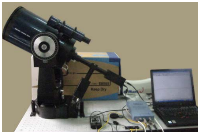
Figure 2. Close-up view of our LIDAR system.
