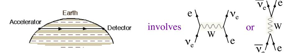
Coherent forward scattering via this W-exchange interaction leads to an extra interaction potential energy —
