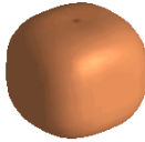
Shape of the heavy hole band energy surfaces in Si
